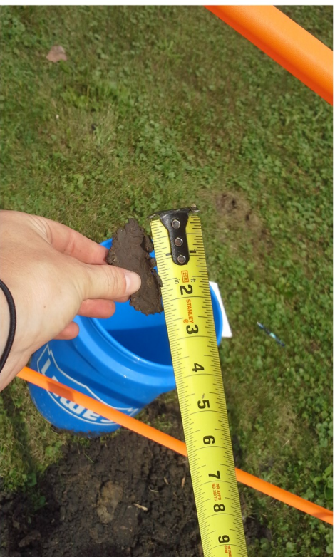
Figure 1. Example of "2-inch + " ribbon of soil at Beraneek Park. This field test can give a comparative indication of clay content in soils. Soil that can be formed into a longer ribbon is likely to have higher clay content than soils that crumble or break off when formed into a ribbon. Higher clay content is often linked to lower percolation rates and slower drainage.
