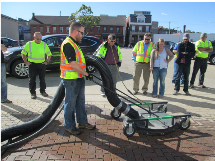
Quick Supply vacuum attachment designed for Pavedrain pavers. Used here on Willow Creek pavers, Dubuque, IA.
